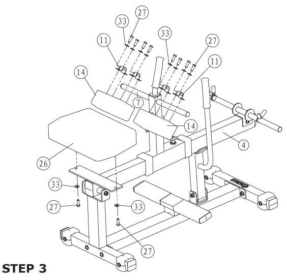
Attach Seat (26) to Swing Frame (4) using: 2 x (27) Bolt 2 x (3 2 x (33) Washer
